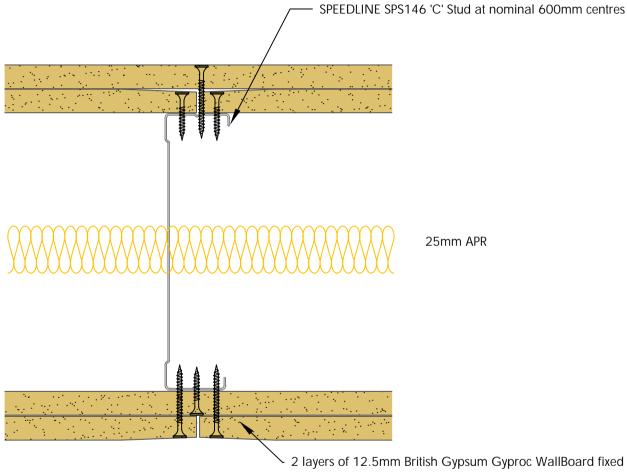
2 layers of 12.5mm British Gypsum Gyproc WallBoard fixed with SPEEDLINE Drywall Screws at 300mm centres (200mm centres at external angles). Ref to table for fixing length.
